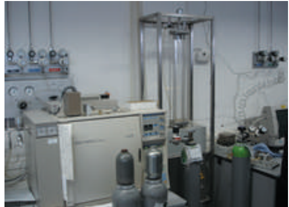
FT-IR spectrometer with long-path cell
