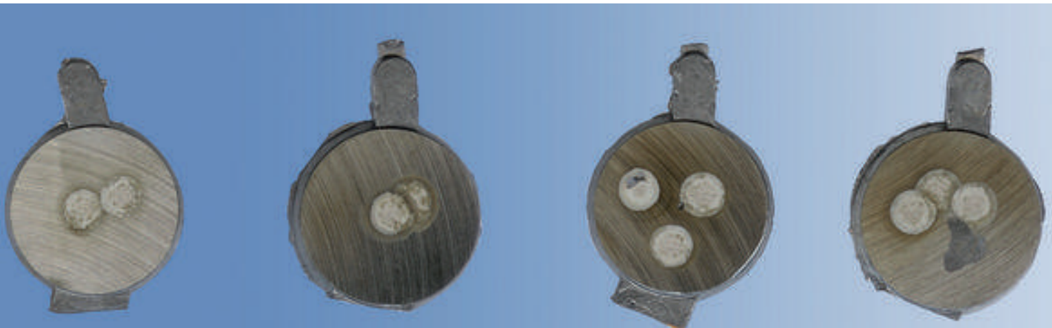
Spark erosion spectrometry: Spots on metallic samples
