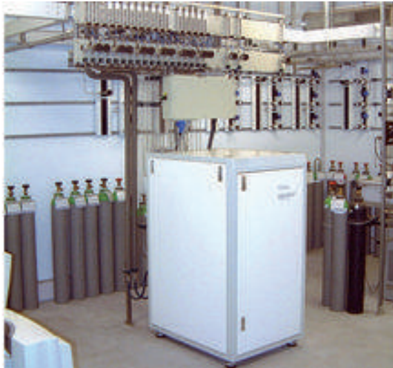
Mass spectrometer for purity analysis of gases
