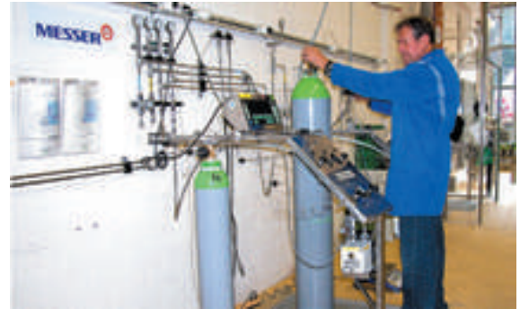
Gravimetric production of high-precision gas mixes
