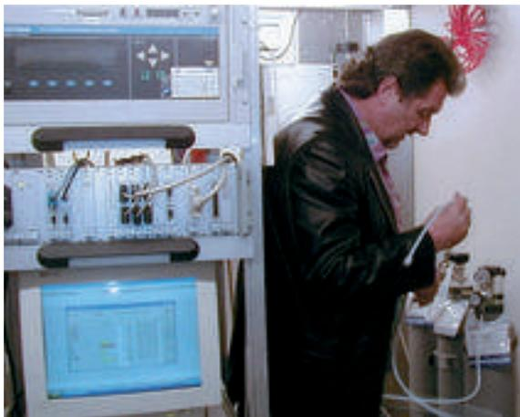
Connecting calibration gases at the measurement station
