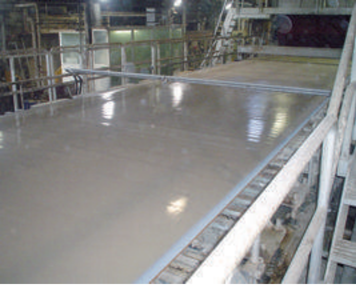
Dewatering of the pigment suspension
