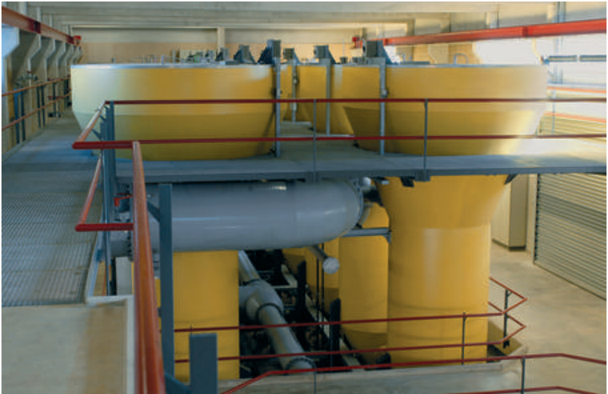
Figure 5: Rapid decarbonization in a fluidized bed with carbon dioxide injection at reactor exit
