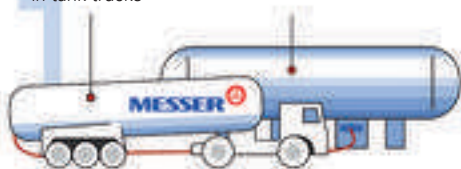
Supply of storage tanks with liquid (CO 2 ) in tank trucks
