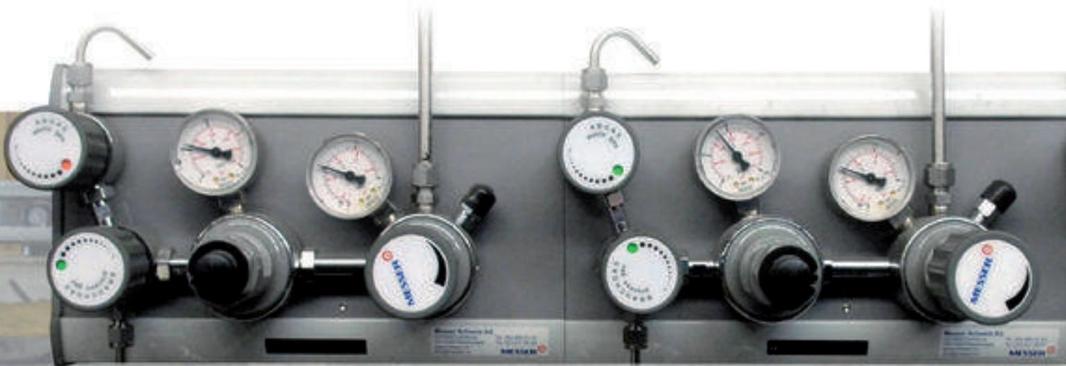
The shielding gas also continuously removes the plasma cloud over the workpiece. The addition of CO<sub>2</sub>, oxygen, helium, nitrogen or hydrogen makes it possible to affect the welding process thermally or metallurgically.
