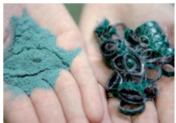
PVC hoses before and after cold grinding
