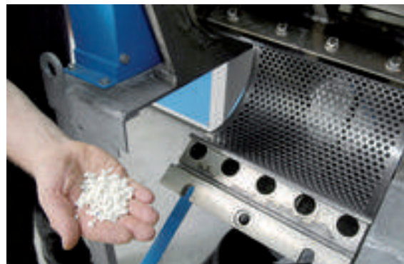
Pre-crushing with cryogenic cutting mill
