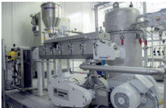
Cryogenic grinding with pin mill
