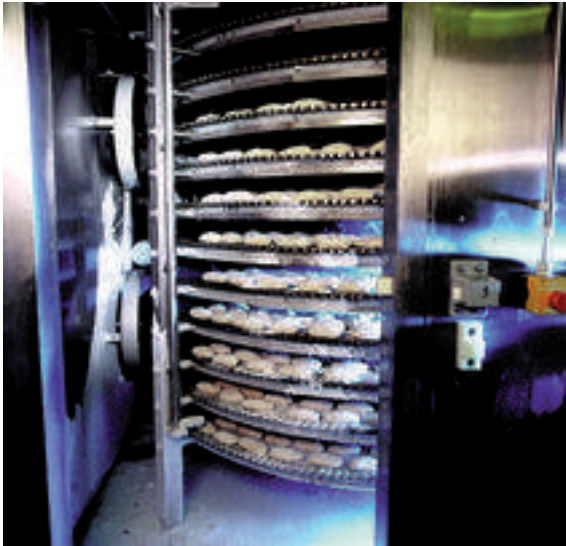
Fig. 7: High freezing capacity in a small area – that's the advantage of the spiral freezer.
