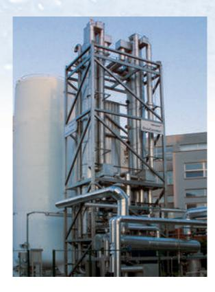
a second downstream condensation stage ensures the recovery of R 12, a pollutant with extremely high vapour pressure which, in ambient conditions, is only present in a gaseous state of aggregation. The evaporating nitrogen in the condensers is used to inert the recycling-machines and thus protect them against dust and pentane explosions.
