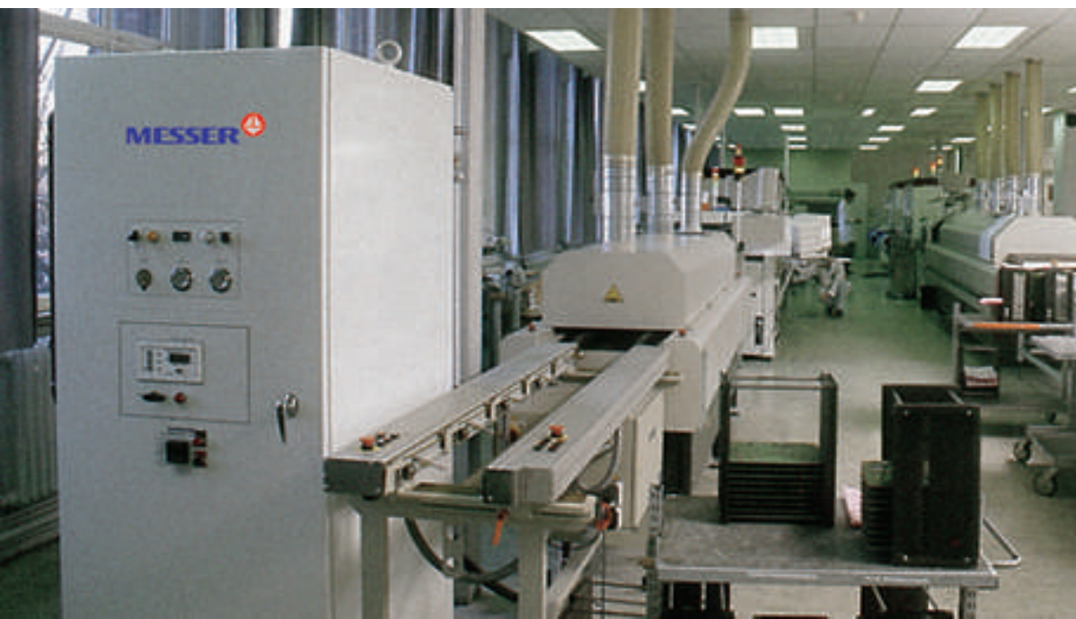
Modern gas-separation technologies such as our membrane systems in compact cabinet enclosures allow cost-effective and user-oriented in-house nitrogen production.
